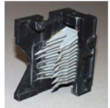
Figure 8: An arc chute assembly
